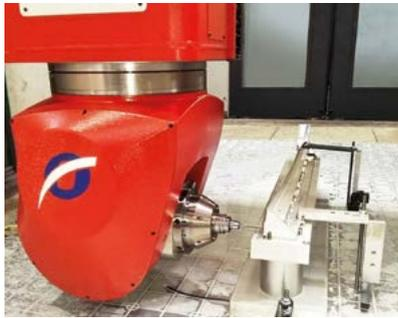
Heidenhain linear scales feedback systems with a 5 micron resolution on the linear axes and highly rigid frames, an enhanced machining accuracy and surface finish quality is achieved.
